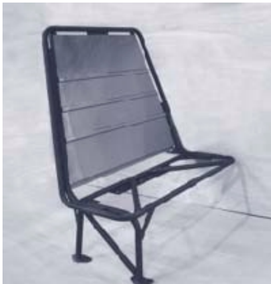
Lap-belt ready seat (note diagonal support and other supporting structure in seat)
